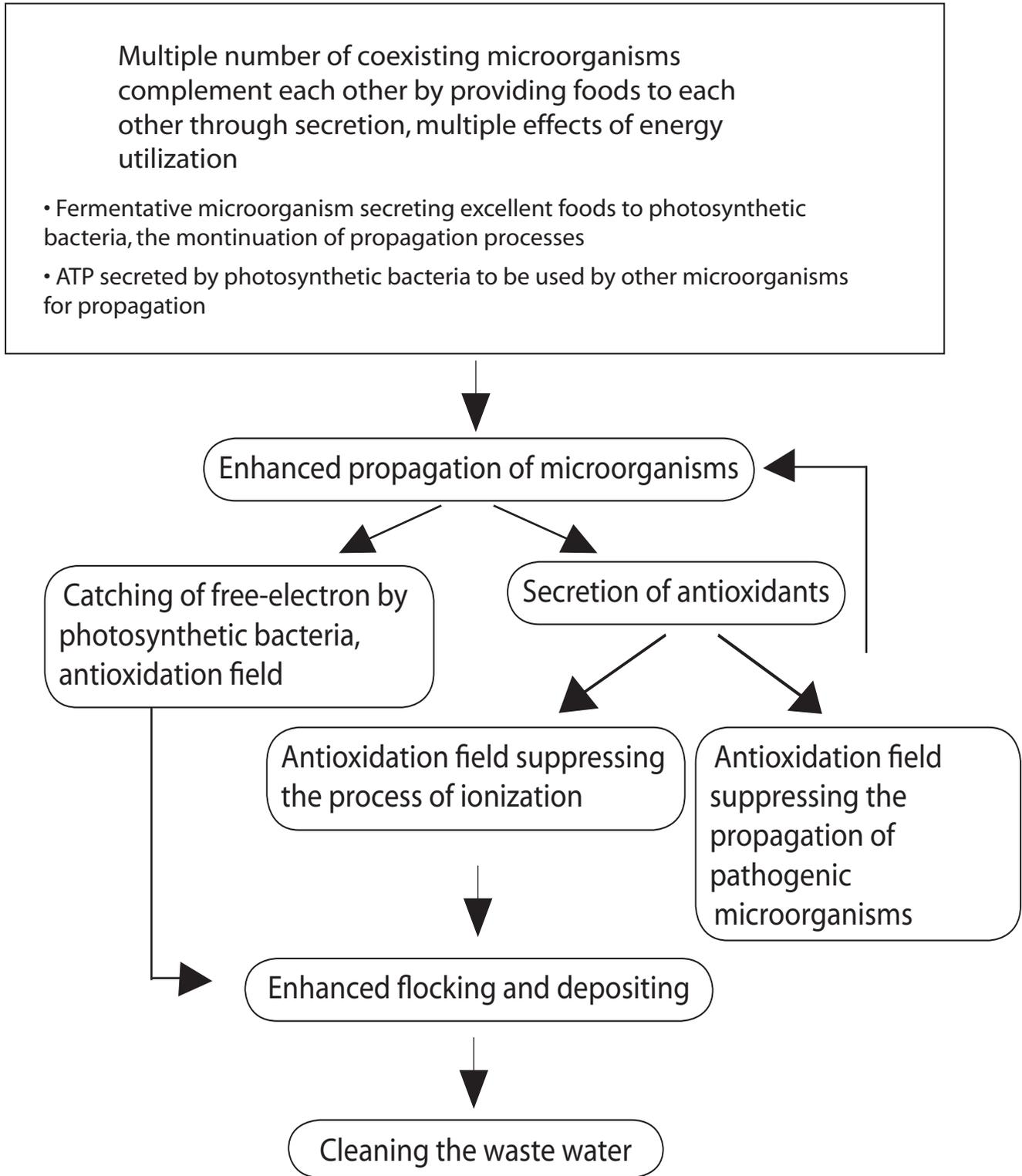
Figure 2-b Natural Oxidation Process
