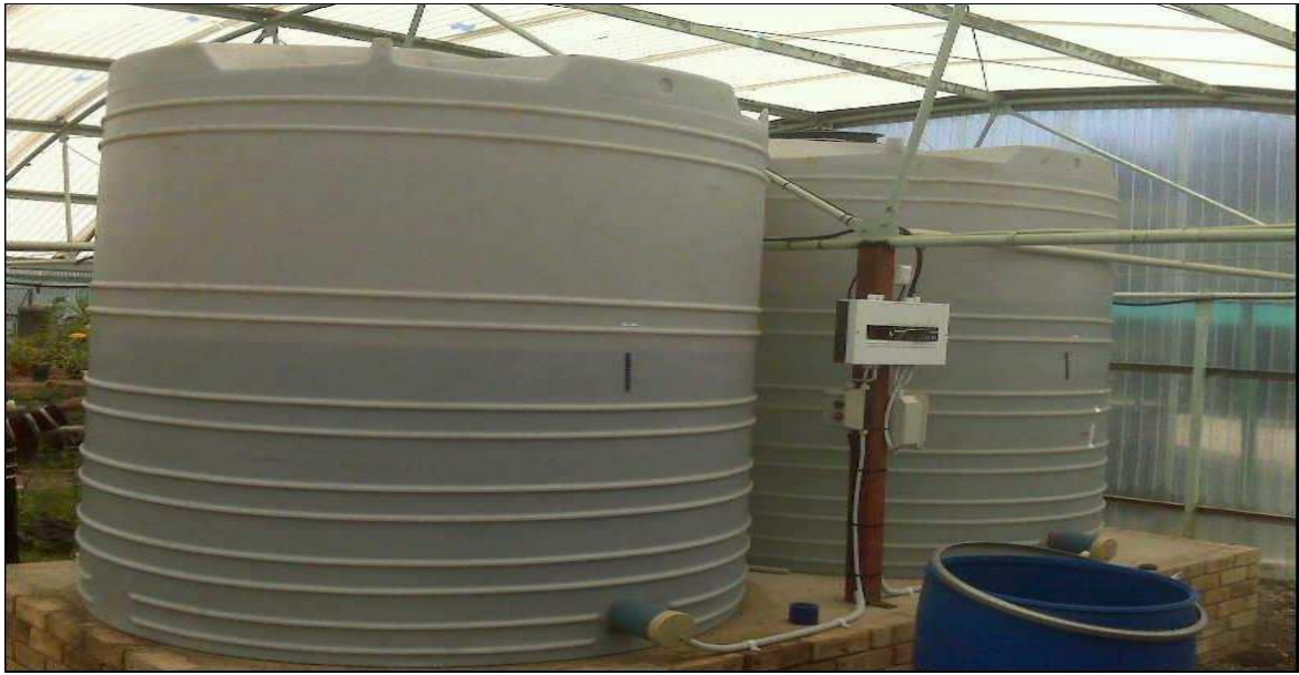
Figure 3.1: The 5000 L tanks used to incubate Multi EM
