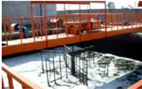
Sprinkling of EM in the equalization tank
