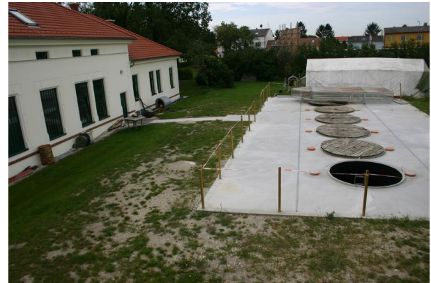
FIG. 1: BOKU experimental site: Quantification of emissions from pilot scale slurry stores with a large open dynamic chamber
